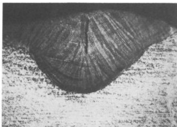
Slika 2 Lita struktura vara z razpokami v toplem Fig. 2 Cast structure of weld with hot cracks
