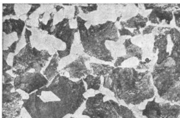
Slika 1 Struktura jekla 1.1 v normaliziranem stanju (500 ×) Fig. 1 Structure of steel 1.1 as normalized (500 ×)
