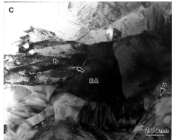
Fig. Plain-view TEM images of the TiC-Fe alloy coatings after heat-treatment
