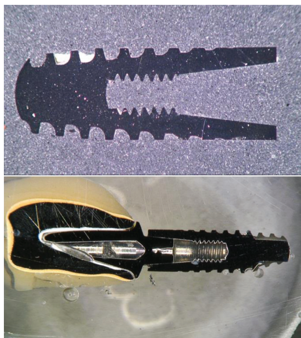
Figure 1: Cross-section of retrieved implant (sample 1) and retrieved dental implant with metal implant abutment and metal ceramic crown (sample 2) recorded with digital microscope Tagarno FHD Trend
