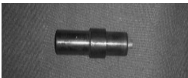
Figure 1: High-carbon high-chromium triangular tool-pin profile
