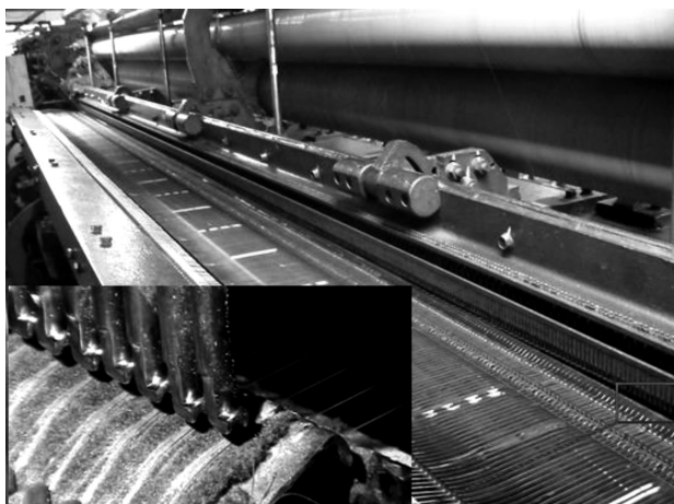
Figure 1: Fishing-net weaving machine and the upper hooks
