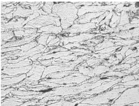
Figure 5: Microstructure of the as-rolled composite with 1.0 % of mass fraction of graphene content after the aging time of 3 h
