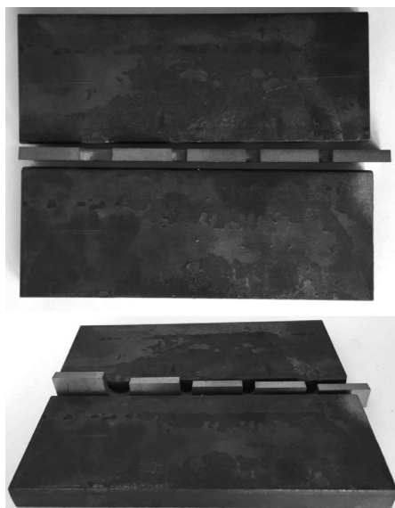
Figure 3: Positions of specimens between holding plates
