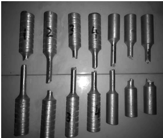
Figure 3: Examined tensile test samples of Al8011 and Al 8011-SiC composites
