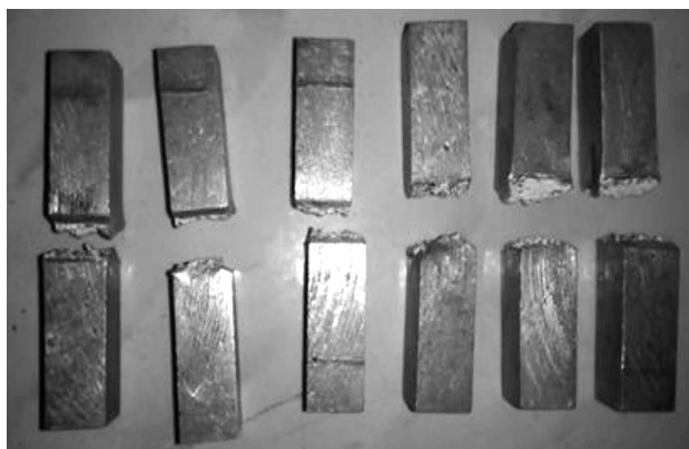
Figure 4: Examined Charpy impact test samples of Al8011 and Al 8011-SiC composites
