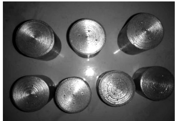
Figure 2: Examined hardness test samples of Al8011 and Al 8011-SiC composites
