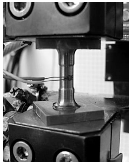
Figure 3: Test specimen in the clamping device of the thermomechanical simulator
