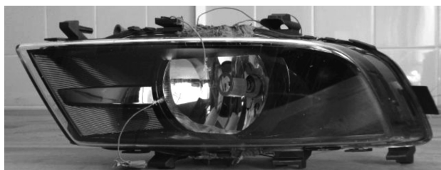
Figure 1: Lamp with thermocouples, front view Slika 1: Žaromet s termoelementi, pogled od spredaj
