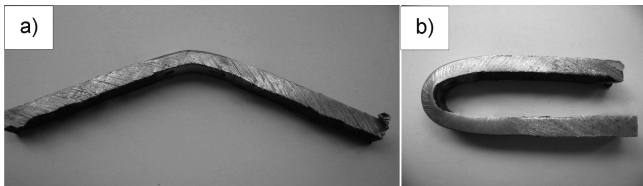
Figure 3: Bending to the first crack: a) specimen 04, b) specimen 531
