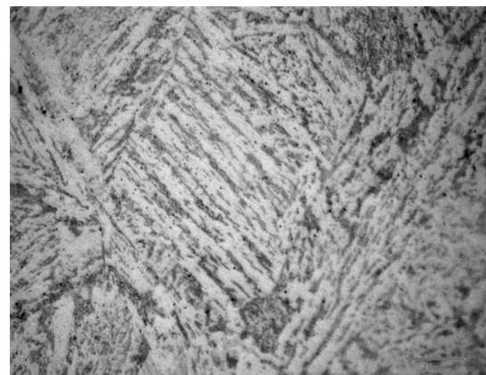
Figure 9: Bainite-ferrite microstructure of the forged part (HV 284) Slika 9: Bainitno-feritna mikrostruktura izkovka (HV 284)
