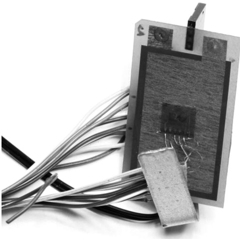
Figure 1: Piezoelectric patch with the applied strain gauges, one on the front side and one on the back side
