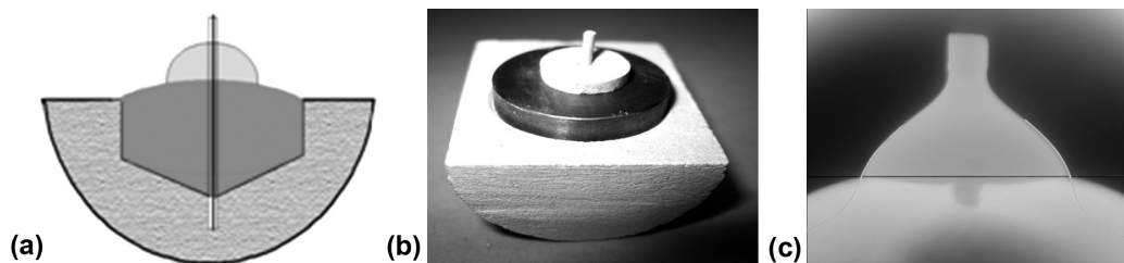
Figure 1: a) Schematic diagram of experimental method, b) a prepared sample before the experiment, c) image of molten phases Slika 1: a) Shematski prikaz eksperimentalne metode, b) pripravljen vzorec pred preizkusom, c) posnetek staljenih faz
