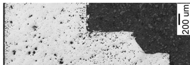
Figure 6: Microstructure of polished bearing B along the ADC direction, snapshot made with MIA technique
