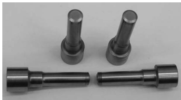
Figure 1: Precracked and fractured V notched cylindrical samples for K_{IC} determination
