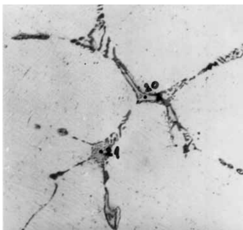
Figure 4: Microstructure of the alloy 1, phases \text{Al}_3\text{Fe} and \text{SnBiAl} . Magn. 730-times
