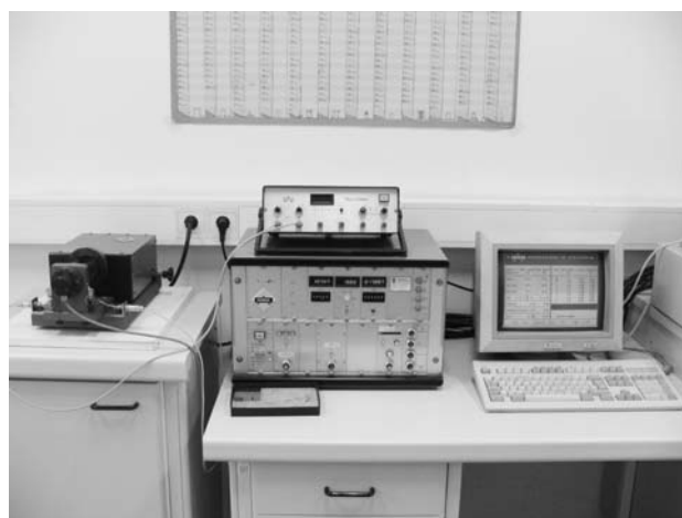
Figure 1: Cracktronic 70 resonant pulsator with the equipment for set up, control, data acquisition, registration and recording of fatigue and crack-growth tests
