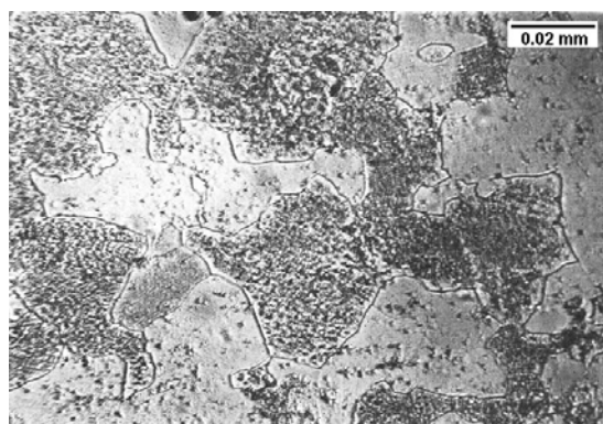
Figure 10: Longitudinal section showing the microstructure after annealing of 100- \mu m-thick foil produced from AA8011 twin-roll cast strip
