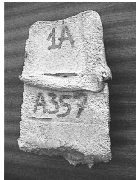
Figure 2: Slurry from A 357 alloy, cut by a knife in the semisolid state
