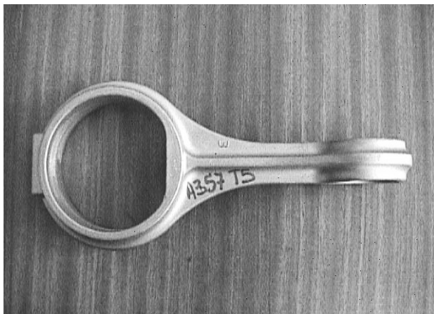
Figure 3: Component 1 (heat treated T5), A 357 alloy Slika 3: Komponenta 1 (toplotno obdelana T5), zlitina A 357
