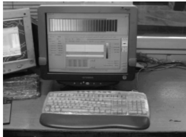
Figure 8: On-line simulation model on the operator desk of the pusher-type furnace
