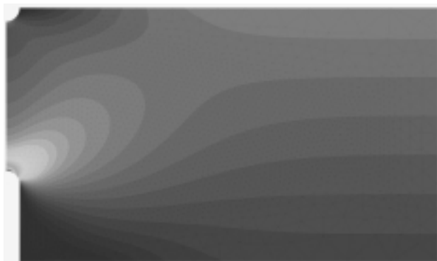
Figure 7: Representation of the horizontal stress distribution in a plate with semi-circular and U-shaped notches
