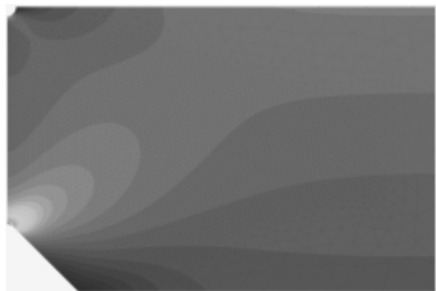
Figure 8: Representation of the horizontal stress distribution in a plate with semi-circular and V-shaped notches
