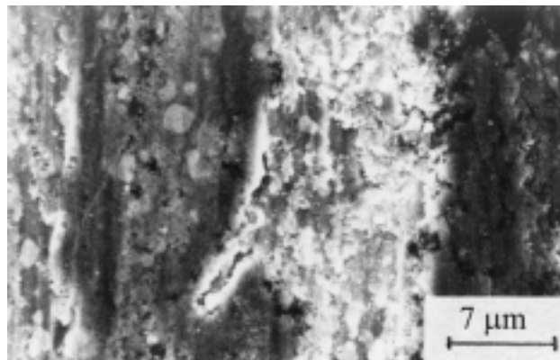
Figure 10: The changes in wear mechanism as a result of increasing testing load, (150 N)
