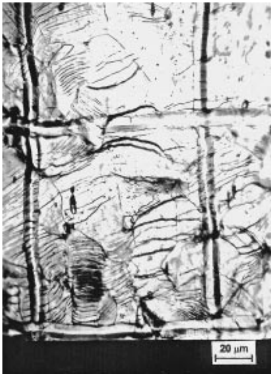
Figure 7: Microstructure of a low carbon steel after static elongation 10% in tension
