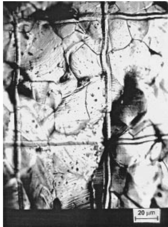
Figure 8: Microstructure of a low carbon steel after dynamic elongation 10% in tension
