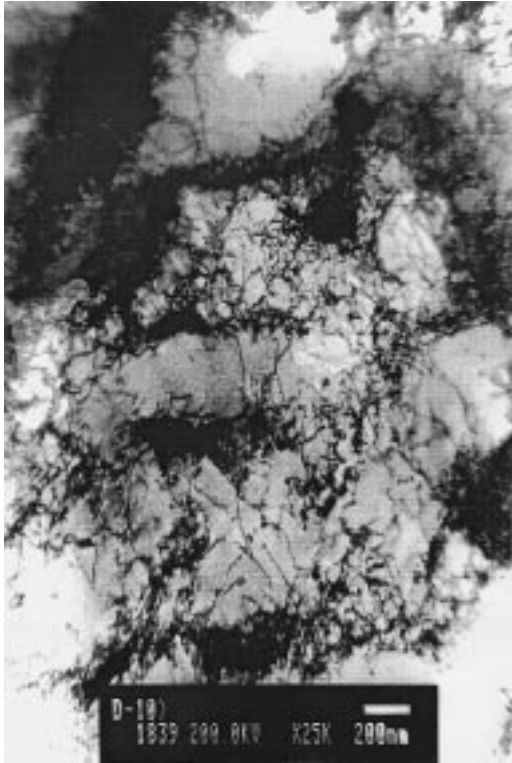
Figure 6: Substructure of a low carbon steel after dynamic elongation 10% in tension
