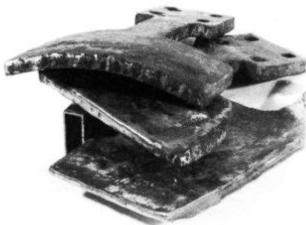
Slika 3: Videz navarjenih robov lopatic in strgala (spodaj) Figure 3: Appearance of surfaced blade edges and scraper edges (below)
