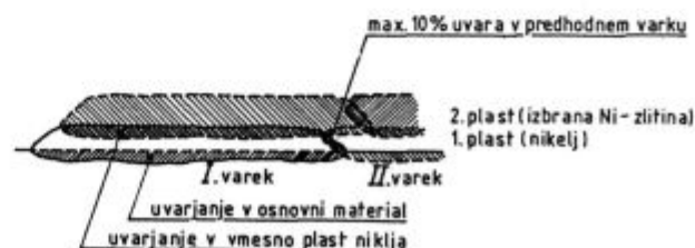
Slika 3: Shema navarjanja ploskev z večžično elektrodo pod legiranimi aglomeriranimi praški Figure 3: Scheme of submerged arc surfacing of a surface with multiple-wire electrode and with alloyed agglomerated fluxes
