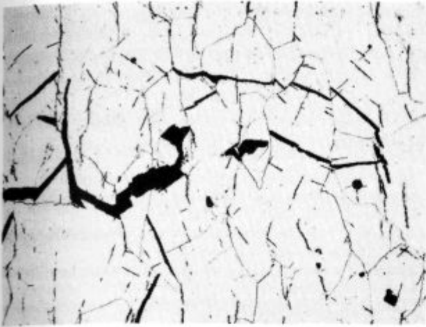
Slika 3: Smeri prelomov se ujemajo z usmerjenostjo karbidov v posameznih zrnih (x 200) Figure 3: Directions of cracks correspond with orientation of carbide needles within each grain (x 200)
