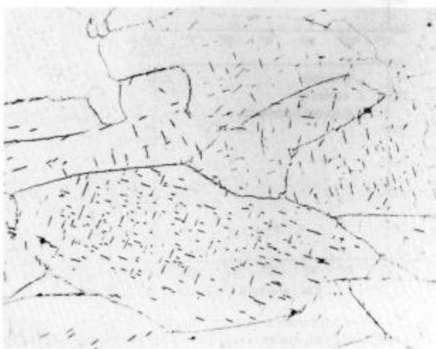
Slika 2: Izločeni karbidi v TVT (x 200) Figure 2: Precipitated carbides in hot rolled strip (x 200)
