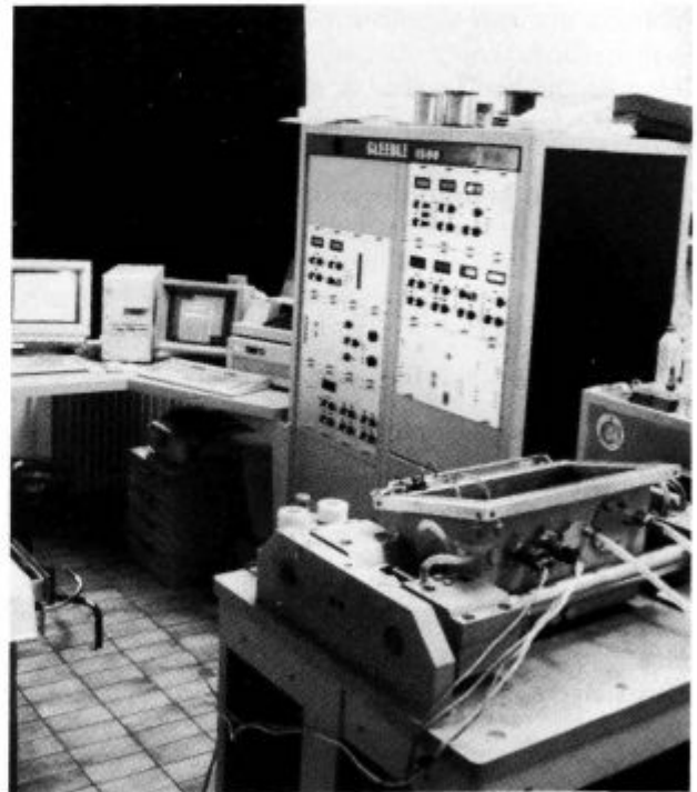
Slika 1: Fizikalni simulator Gleeble 1500. Termalni sistem omogoča hitrost segrevanja od 0.1 do 10000 K/s, hitrost ohlajanja do 1000 K/s. Mehanski sistem zagotavlja hitrost pomika bata od 0.000017 do 2000 mm/s, hitrost naraščanja sile od 0.001 do 200 kN/s oziroma hitrost deformacije od 0.0001 do 50/sek pri tlačnih in 70/s pri nateznih testih Figure 1: Physical simulator Gleeble 1500. Thermal system allows heating rates from 0.1 up to 10000 K/sec, cooling rates up to 1000 K/sec. Mechanical system enables piston rates from 0.000017 to 2000 mm/sec, force rates from 0.001 to 200 kN/sec that allow strain rates from 0.001 to 50/sec using compression test and from 0.001 to 70/sec using tension test
