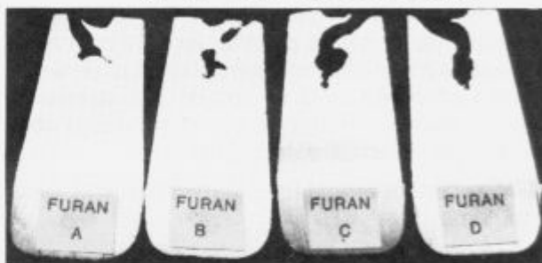
Figure 2. Sections of three samples, cast in different sand moulds; ratio M_{fn}/M_c = 0.25 , unalloyed ductile cast iron.
