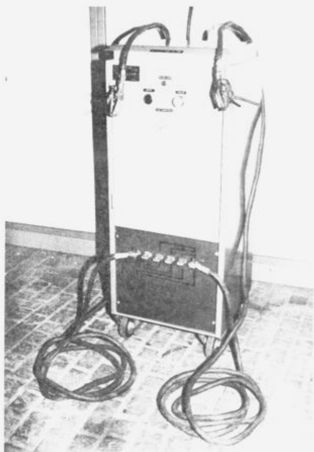
Slika 5. Naprava za žarjenje koncev vlečene žice. Figure 5. Equipment for conduction annealing of cold drawn wire ends.
